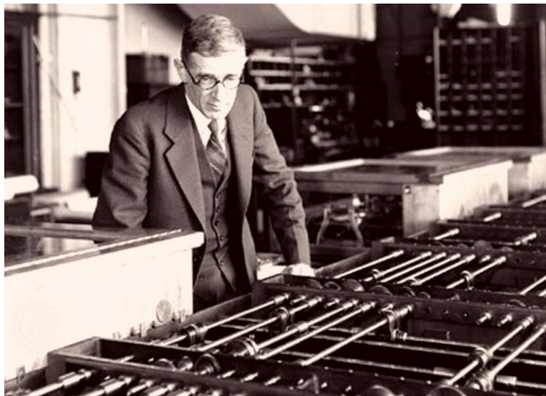
Bush testing out the Profile Tracer, his first machine, built in his engineering doctorate program. It formed the basis for his next invention.
